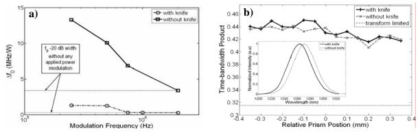
**Fig.2:** a) frequency response of  $f_0$  width to fast power modulation with (dotted) and without (solid) the knife edge. b) Time-bandwidth product for our Cr:f laser with (thick dotted) and without (thick solid) the knife edge inserted compared to the transform limited case (narrow dotted), inset shows the difference in the power spectra with (solid) and without (dotted) the knife edge inserted.
