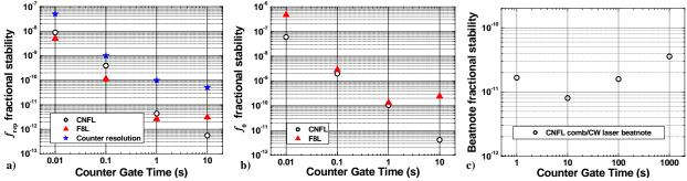
Fig. 2:The CNFL  $f_{rep}$  and  $f_0$  fractional stability compared with those of our F8L laser. a) The  $f_{rep}$  fractional stability, which is beyond the Rb GPS specification. b) The  $f_0$  fractional stability. The CNFL comb shows a comparable fractional stability to the F8L comb. c) The fractional stability of the beat between an acetylene stabilized CW laser against the CNFL comb.
