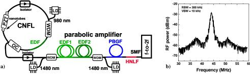
Fig. 1: a) The phase-stabilized carbon nanotube fiber laser comb generator. LD: laser diode; OC: output coupler; WDM: wavelength division multiplier; PBGF: hollow core photonic bandgap fiber; SMF: single mode fiber. b) The carrier envelope offset frequency was measured by the f-to-2f interferometer with a 1 MHz width (FWHM), resolution bandwidth (RBW) of 300 kHz.
