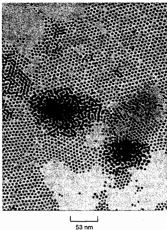
Figure 5. Segregation of different size nanocrystals on a TEM grid due to the decrease of colloid temperature.
