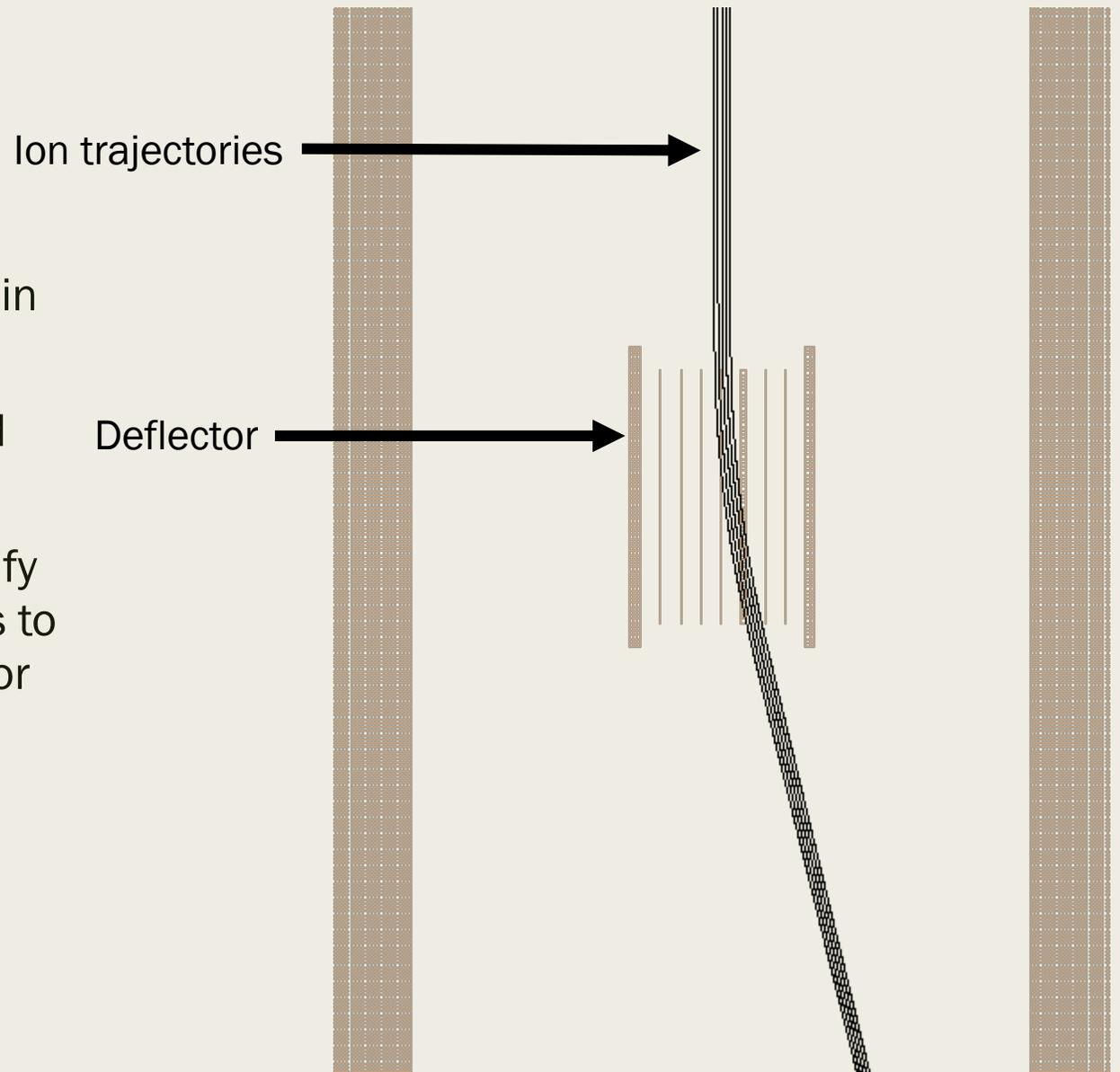
Example of an ion trajectory in Simion
