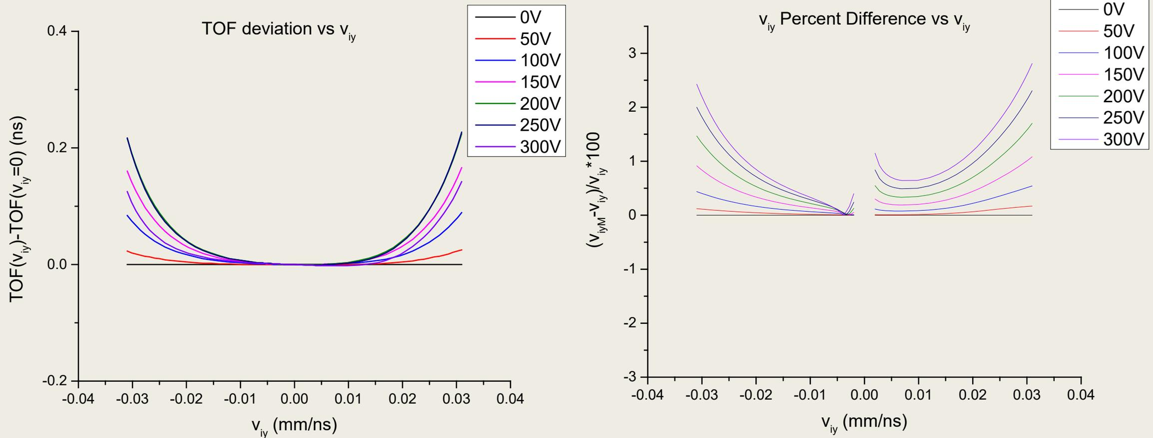
For  $v_{ey}$  less than 5 eV, TOF deviation is less than 0.2 ns. The time resolution of our setup is 0.2 ns.
