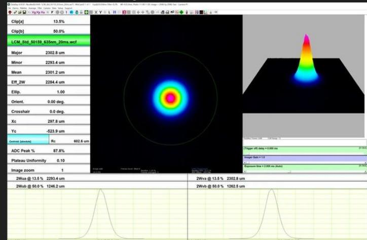
DataRay Visible Laser Beam Profiling
