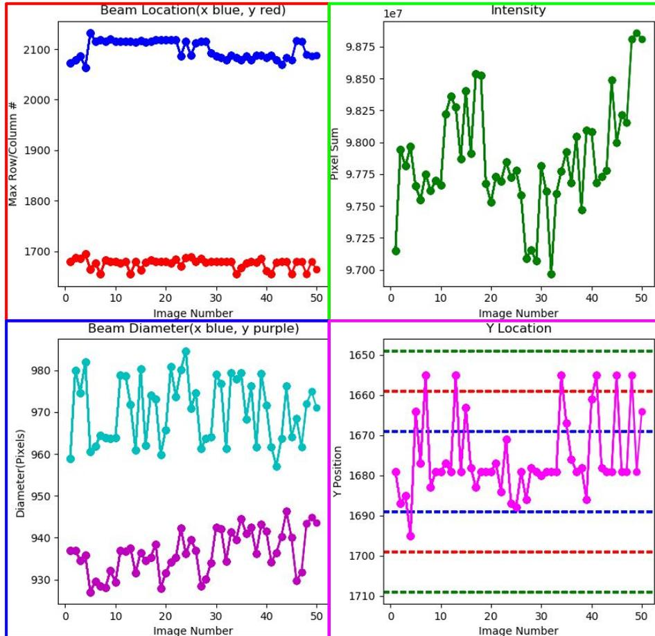
1. Shows broad view of vertical and horizontal position, same type of plot as the exaggerated beam walk plot.
