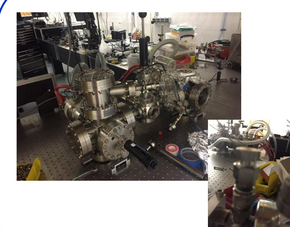
The high harmonic chamber consists of two pumping differential chambers that are connected to two turbo pumps. These turbo pumps allow the pressure to stay constant at 10<sup>-6</sup> torr. This pressure is needed to keep ambient air out of the chamber and only allow argon gas, the non-linear medium, to be ionized. The pressure is also needed to be low so that the MCP does not become defective and break when exposed to the water vapor present in ambient air.
