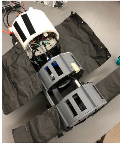
Another view of the completed instrument showing the anodised aluminum foil light shades folded out.
